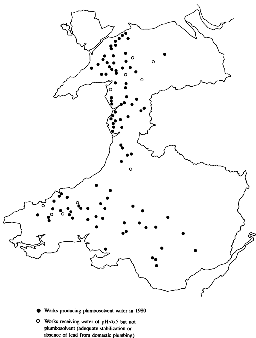
Fig. 9.1. Water-treatment works supplying plumbo solvent and aggressive water.
